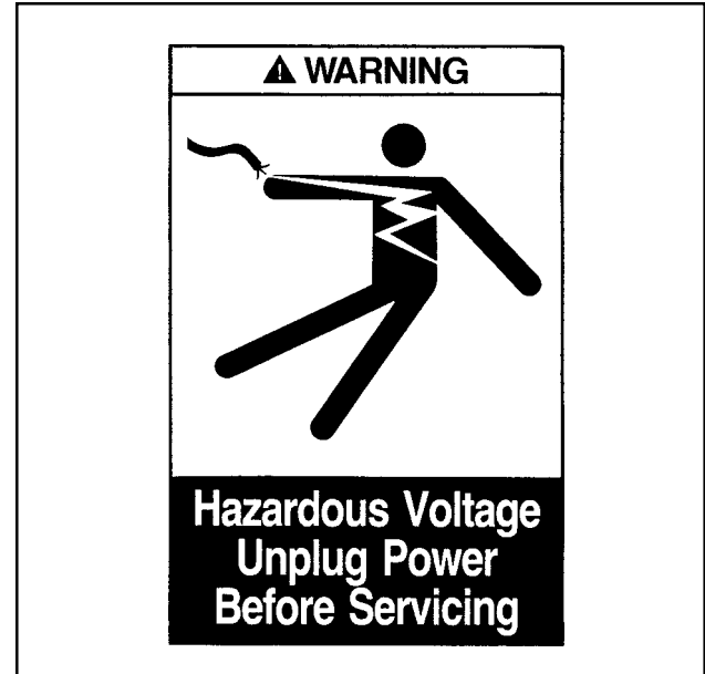
Figure 1-2 – Electrical Warning Label
