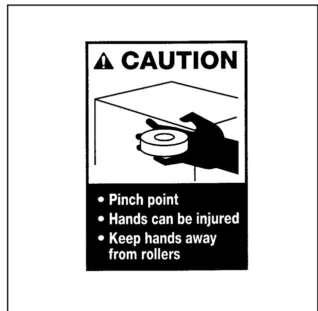
Figure 1-3 – Pinch Point Caution Label
